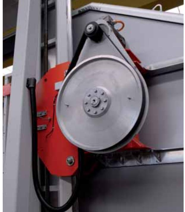
*The driving wheel is driven by a belts/pulleys system and by an inverter controlled motor to manage the diamond wire peripheral speed.*
