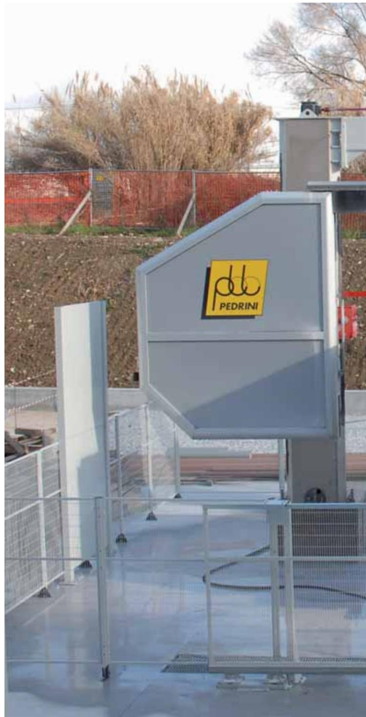
*Pedri SINGLEWIRE JUPITER GS210 performs single cuts on marble, granite and natural stones blocks up to 4200 mm long. It can be used both for squaring and for cutting blocks into slabs.*
